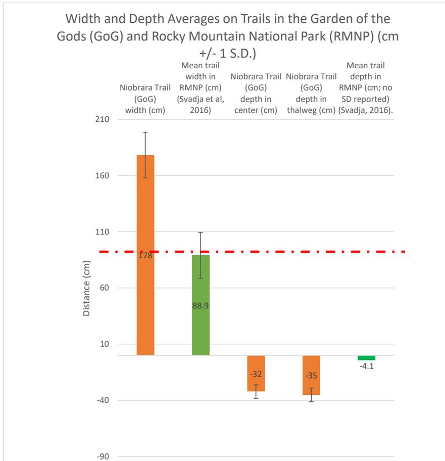
Figure 2. Trail depth measurements are presented as negative numbers because they are below the level trail surface from which the trail width measurements are taken. The Niobrara trail (179cm +/- 20cm) has nearly twice the average trail width measured in RMNP and twice the maximum tread width specified in the Super Friends Trail Standards Agreement (2017), which is indicated by the red dashed line at 91 cm. The Niobrara trail is also deeply incised with an average depth of 35 cm (+/- 6cm).
