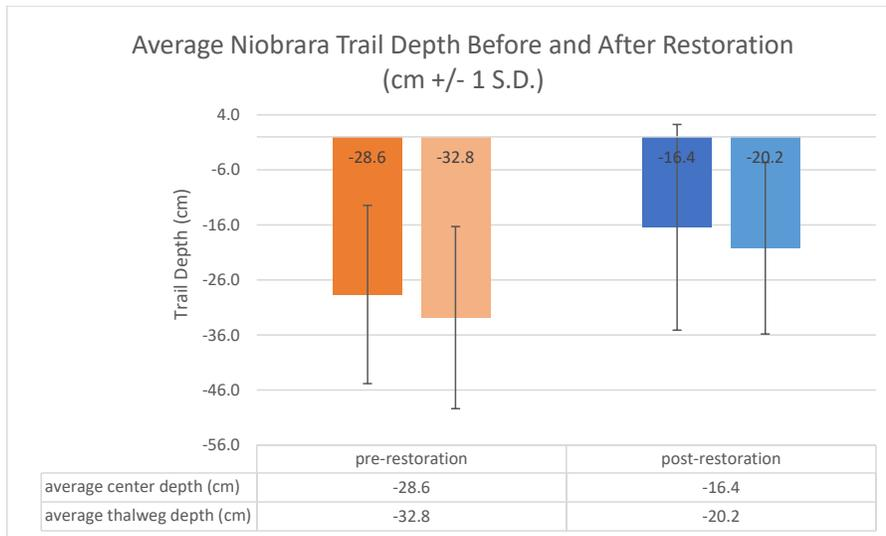
Figure 6. Although the thalweg depth and center depth measurements are not significantly different, the relative change before and after restoration are notable as convergence in these measurements indicates a more level trail, which is a goal of the restoration efforts.
